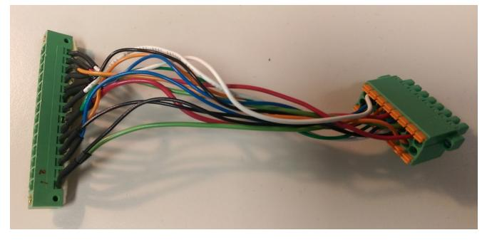
(from left to right) 9900/9900+ GPIO connector plugs in here, then dual-row F800 connector plugs into F800 GPIO
